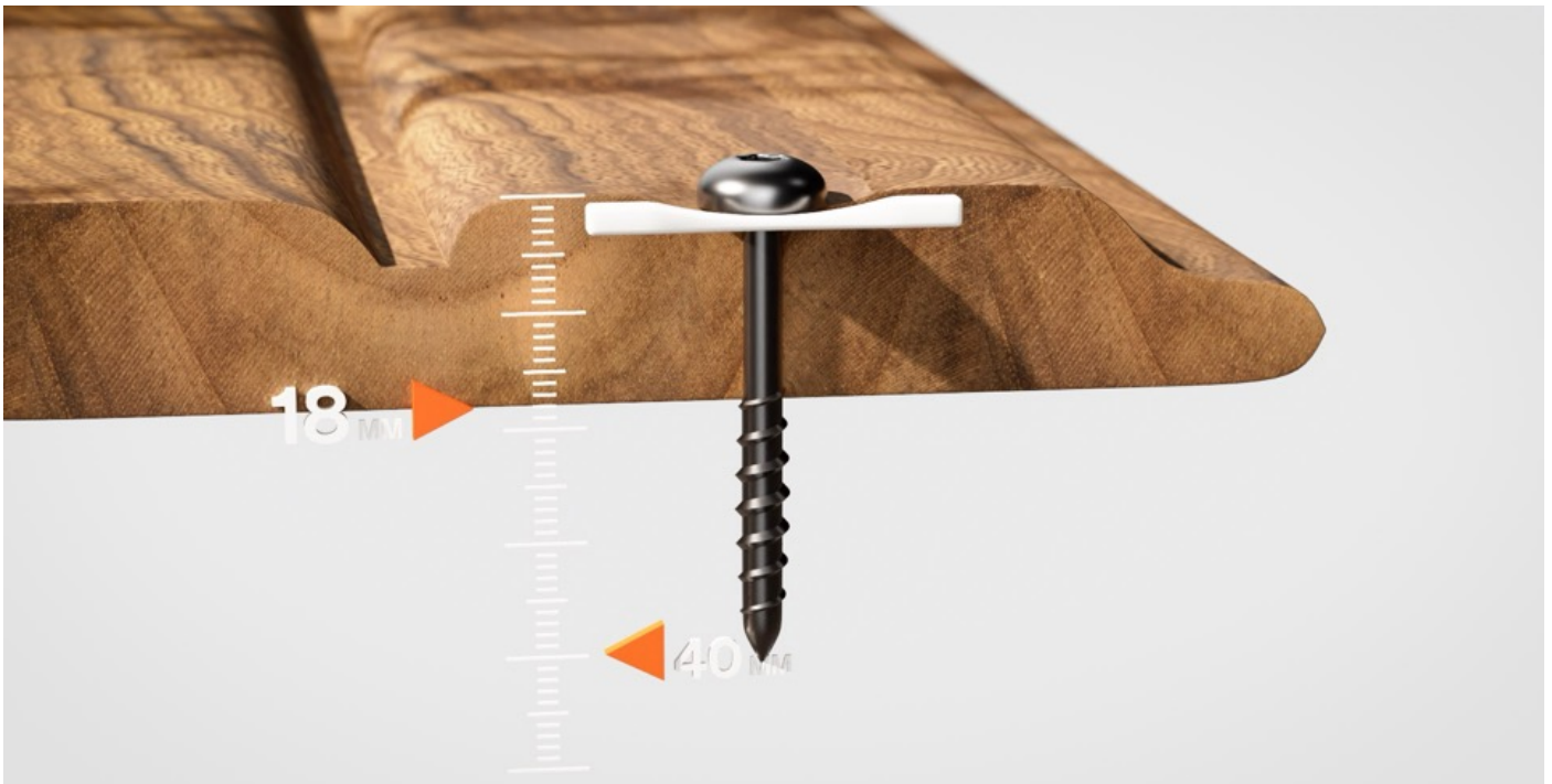
Image 7: Do not drive or screw fasteners below the surface of the wood, to prevent water ingress
