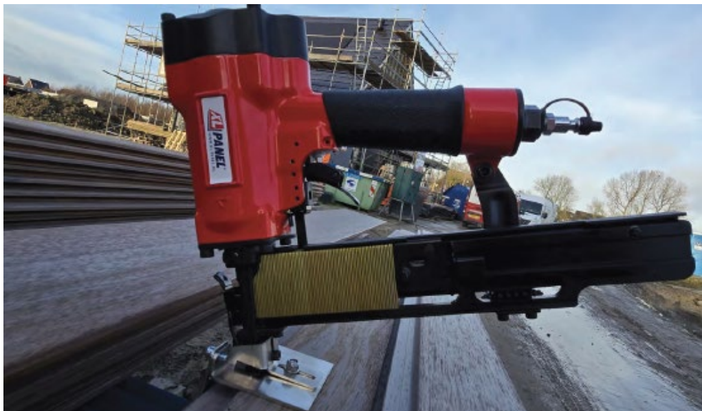
Image 2: Staple gun with attachment developed by XL-Panel
