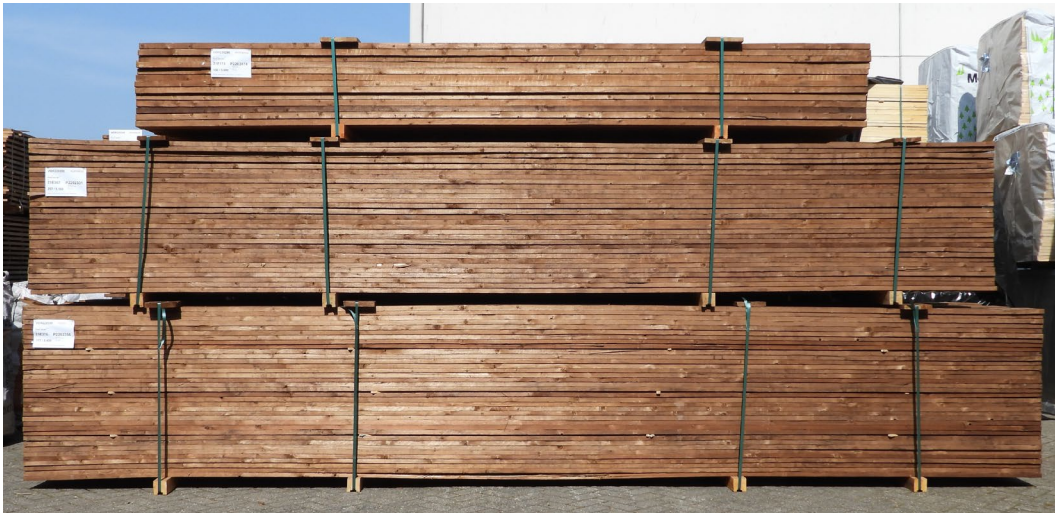
Figure 1 - Store untreated wood in the correct way
