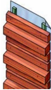
Figure 3 - Horizontal open cladding with variable dimensions, trapezoidal for proper drainage.
