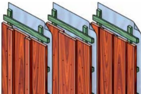
Figure 4 - Vertical cladding From left to right: cover boarding, cover boarding and rabate with half-lap overlap (channelsiding).
